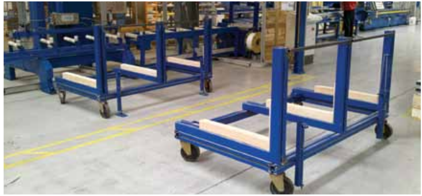
Stud and Track - two trolley system (see point 12 below)
