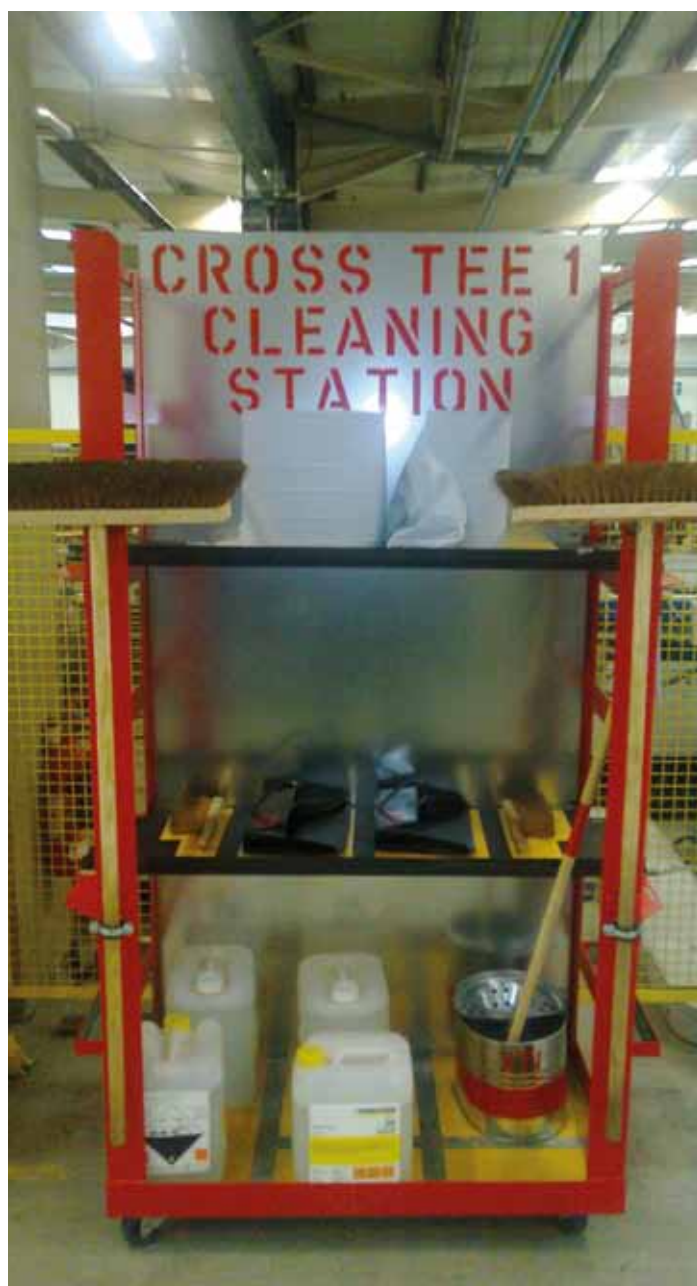
A 5S cleaning station. SAS has manufactured one for each of the lines in the Roll Form department – they hold all the equipment operators need to carry out their daily clean down routine.
