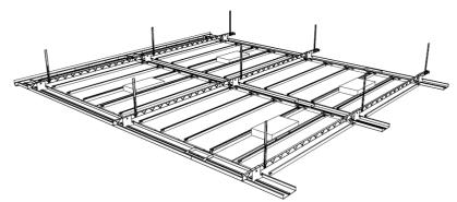
**SAS330** is a lay-in suspended steel ceiling system; it offers the facility to design the ceiling to any building grid size. Tiles are available in a range of shapes and sizes to meet individual project requirements. A range of acoustic backing options provide up to 49dB acoustic attenuation or Class A acoustic absorption. For further details please visit <a href="https://sasintgroup.com/metal-ceilings/suspended-sas330/">https://sasintgroup.com/metal-ceilings/suspended-sas330/</a>
