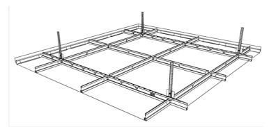
**SAS130** is a modular lay-in steel ceiling system; tiles are supported from SAS Alugrid or SAS Tee Grid. Alugrid-Q features a continuous linear recess with an M6 thread while providing a completely flush ceiling. Alugrid-P is a plain version without the threaded recess; Tee Grid provides a tegular effect. A range of acoustic backing options provide up to 45dB acoustic attenuation or Class A acoustic absorption.
