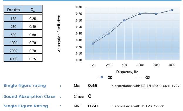
During testing, absorption coefficients occasionally reach values greater than unity. Theoretically this is impossible by definition. These anomalies occur due to diffraction of the impinging sound waves at the edges of the test samples. In practical terms this is insignificant. Absorption coefficients greater than unity are assumed to be unity and reported as such.
