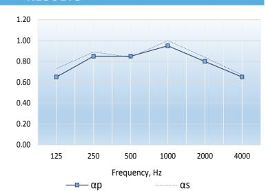
Single figure rating :  $\Omega \omega$  0.80(L) In accordance with BS EN ISO 11654: 1997
